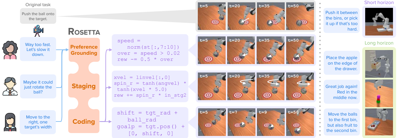
Fig. 1: ROSETTA’s three-module structure takes unconstrained, unseen natural language preference and generates reward code that incentivizes desired behavior. ROSETTA can adapt to diverse behavioral preferences, not only in position but orientation and speed. We validate ROSETTA’s performance in two short-horizon and three long-horizon task-agnostic environments.
