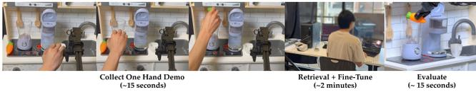
Fig. 10: **Fast Adaptation.** We conduct a small-scale user study to demonstrate HAND’s ability to learn robot policies in real-time. From providing the hand demonstration (Left), to retrieval and fine-tuning a base policy (Middle), to evaluating the policy (Right), we show that HAND can learn to solve the Blend Carrot task with 7.5/10 task completion in less than 3 minutes
